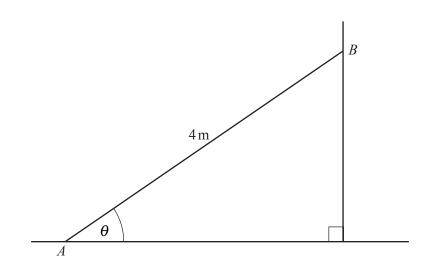
A uniform ladder *AB* of weight *W*N and length 4 m rests with its end *A* on rough horizontal ground and its end *B* against a smooth vertical wall. The ladder is inclined at an angle  $\theta$  to the horizontal where  $\tan \theta = \frac{1}{2}$  (see diagram). A small object *S* of weight 2*W*N is placed on the ladder at a point *C*, which is 1 m from *A*. The coefficient of friction between the ladder and the ground is  $\mu$  and the system is in limiting equilibrium.
